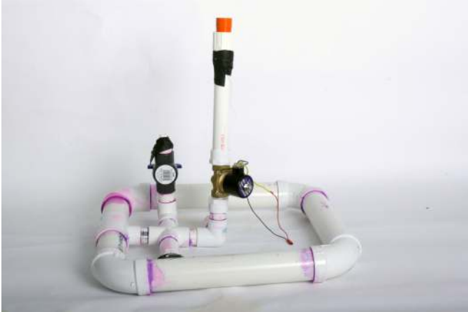
Fig. 4: SnotShot . When the pressurized air is released, the vertical reservoir of analogue snot is expelled from the 3D-printed blowhole, pictured in orange.
