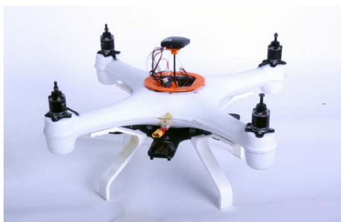
Fig. 1: SnotBot “White” is a modified Aquacopter Project X Quadcopter Frame . The chassis is completely waterproof, leaving only the motors, propellers, and waterproofed batteries exposed. Olin students modified it to include a landing structure, attachment points for a bottom-mounted camera, and robust internal electronics support structure. This is just one of several vehicles in the current fleet.
