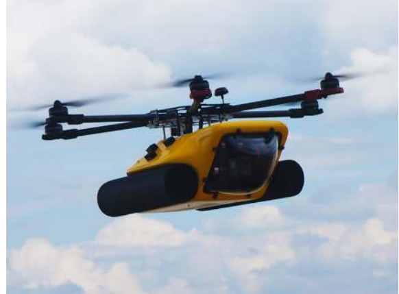
Fig. 3: A representative picture of the new fleet hexacopters, which are a pair of recently acquired HexH2Os produced by QuadH2O multirotors . Picture courtesy of QuadH2O website, http://www.quadh2o.com .
