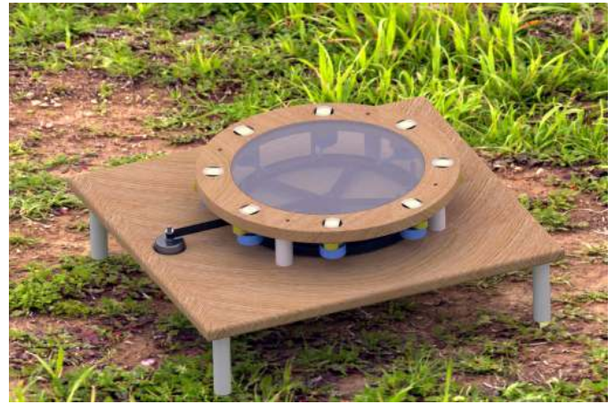
Fig. 5: A representative render produced in SolidWorks of the launch and recovery platform. MagSwitches will be used to catch the bottom of the landing structure of a SnotBot during landing, and can be turned off for launch.
